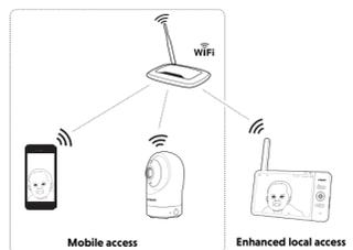
If you want to stream live video remotely with your mobile device, download and install the **MyVtech Baby Pro** mobile app. With the mobile app, your Wi-Fi router (not included) provides Internet connectivity to your HD video monitor system. It serves as a communicating channel between your baby unit and mobile device, allowing you to monitor and/or control your baby unit wherever you are. For more details, see **Download app for mobile access** section in this quick start guide.
