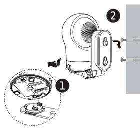
5. You can maximise your baby unit's viewing angles by tilting the wall mount bracket. Hold the baby unit, and then rotate the knob in an anticlockwise direction. This will loosen the joint of the wall mount bracket. Tilt your baby unit up or down to adjust to your preferred angle. Then, rotate the knob in a clockwise direction to tighten the joint and secure the angle.
