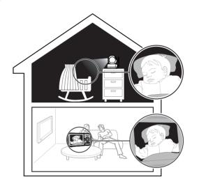
The baby unit has infrared LEDs that allow you to see your baby clearly at night or in a dark room. When the baby unit being viewed detects low light levels, the infrared LEDs are switched on automatically. The images from the baby unit are in black and white, and 🥝 appears on the screen.
