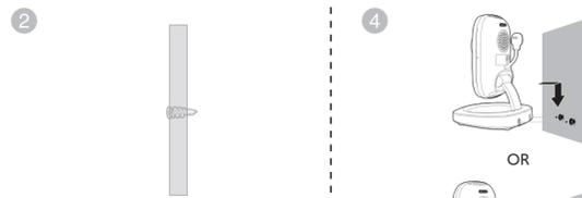
Drill two holes in the wall. If you drill the holes into a stud, go to step 3.
