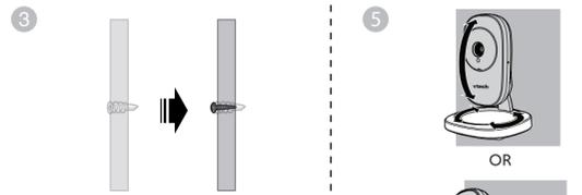
Insert the screws into the holes and tighten the screws until only 6mm of the screws are exposed.
