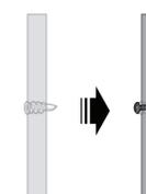
Insert the screws into the holes and tighten the screws until only 6mm of the screws are exposed.
