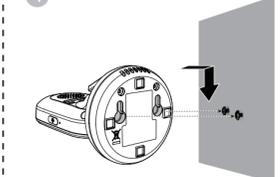
Align the wall mount holes on the baby unit with the screws on the wall. Slide the baby unit down until it locks into place.
