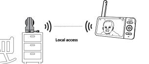
You may experience reduced signal strength if your parent unit and baby unit are far apart, or there are obstructing factors, such as internal walls, between them. Move the parent unit closer to the baby unit to improve the signal strength. You can also set up **Router mode** to connect via your home Wi-Fi network to improve the connection between your parent unit and baby unit
