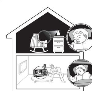
The baby unit has infrared LEDs that allow you to see your baby clearly at night or in a dark room. When the baby unit being viewed detects low light levels, the infrared LEDs are switched on automatically. The images from the baby unit are in black and white, and
